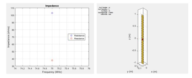
In above example, the dipole is meshed at 75 MHz automatically before calculating the impedance at that value. Use the mesh command to view the meshed dipole. The number of triangles is 44.
