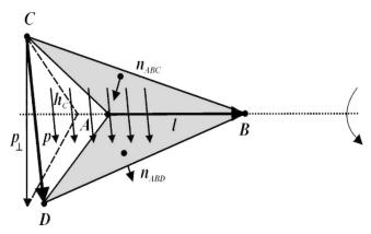
The figure shows an edge-based basis function. The vector variation is perpendicular to the base edge AB (or  $\bar{l}$ ). The vector of the edge CD (or  $\bar{p}$ ) defines the basis function. Within a tetrahedron, the basis function is a constant field given by
