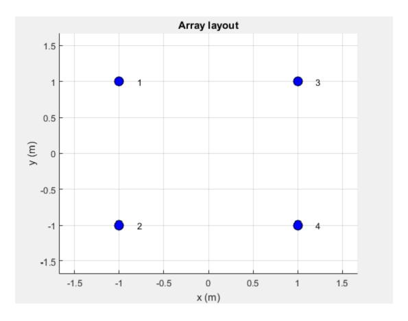
There are four ports in this array. The corresponding S-parameter matrix would be of size  $4 \times 4$ :
