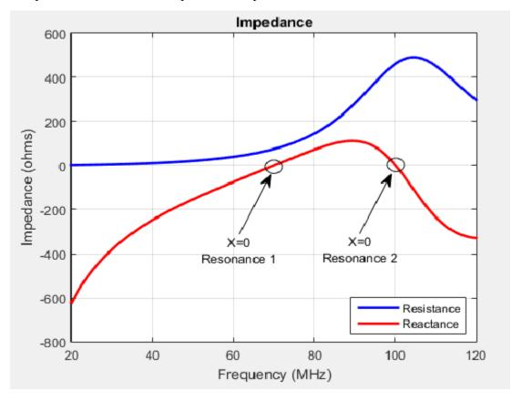
In the plot, the reactance values are negative, or capacitive, before the resonance. These values are positive or inductive after the resonance. This type of resonance is called series resonance. You can model this type of resonance using a series RLC circuit. If the impedance curve goes from positive reactance to negative reactance, it is called parallel resonance. You can model this type of resonance using a parallel RLC circuit.
