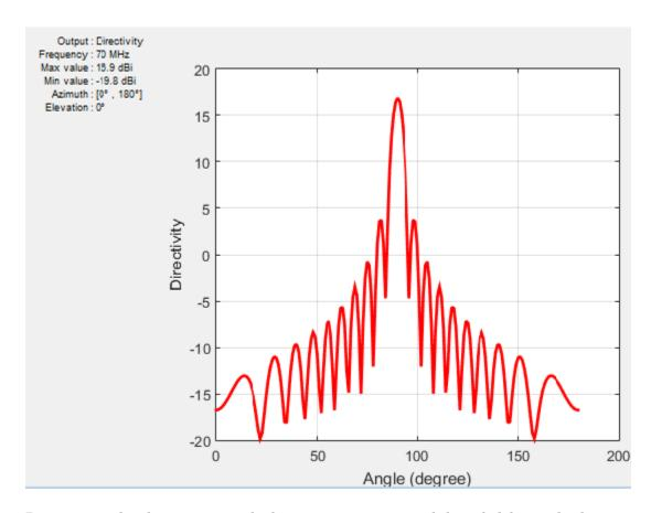
By using amplitude tapering on the linear array, you control the side lobes and achieve a better main beam in the desired direction:
