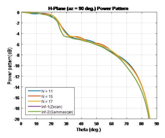
For finite arrays of size greater than 10 x 10, the scan element patterns in the E-, D-, and H-planes match the patterns of the infinite array scan element.
