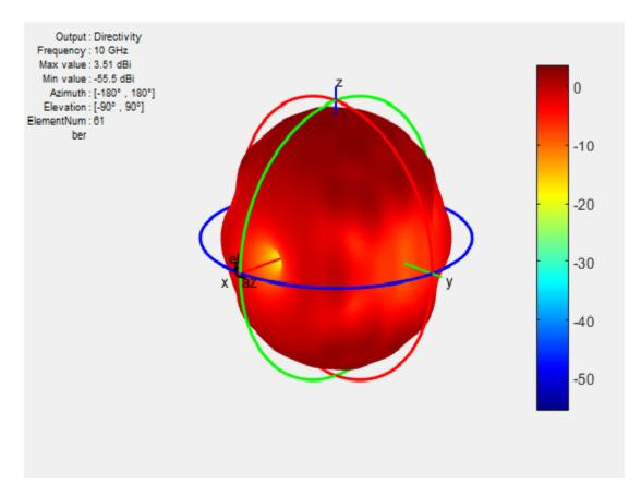
The figure shows the embedded element pattern of a center element in a 11x11 array. You can also calculate the embedded element pattern as a magnitude of electric field.
