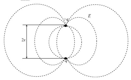
If you place a conducting object along this equipotential surface, then the field above the surface does not change.
